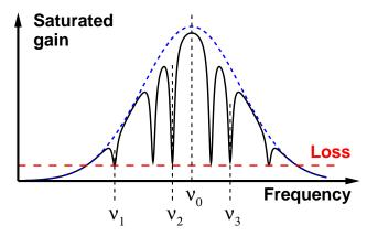
The system displayed in the figure is oscillating on the 3 frequencies  $v_1$ ,  $v_2$  and  $v_3$  and digs 6 holes into the profile including the mirror holes. The relative intensities are given by hole area ratioes. Higher order transverse modes are assumed suppressed with mode selective losses.
